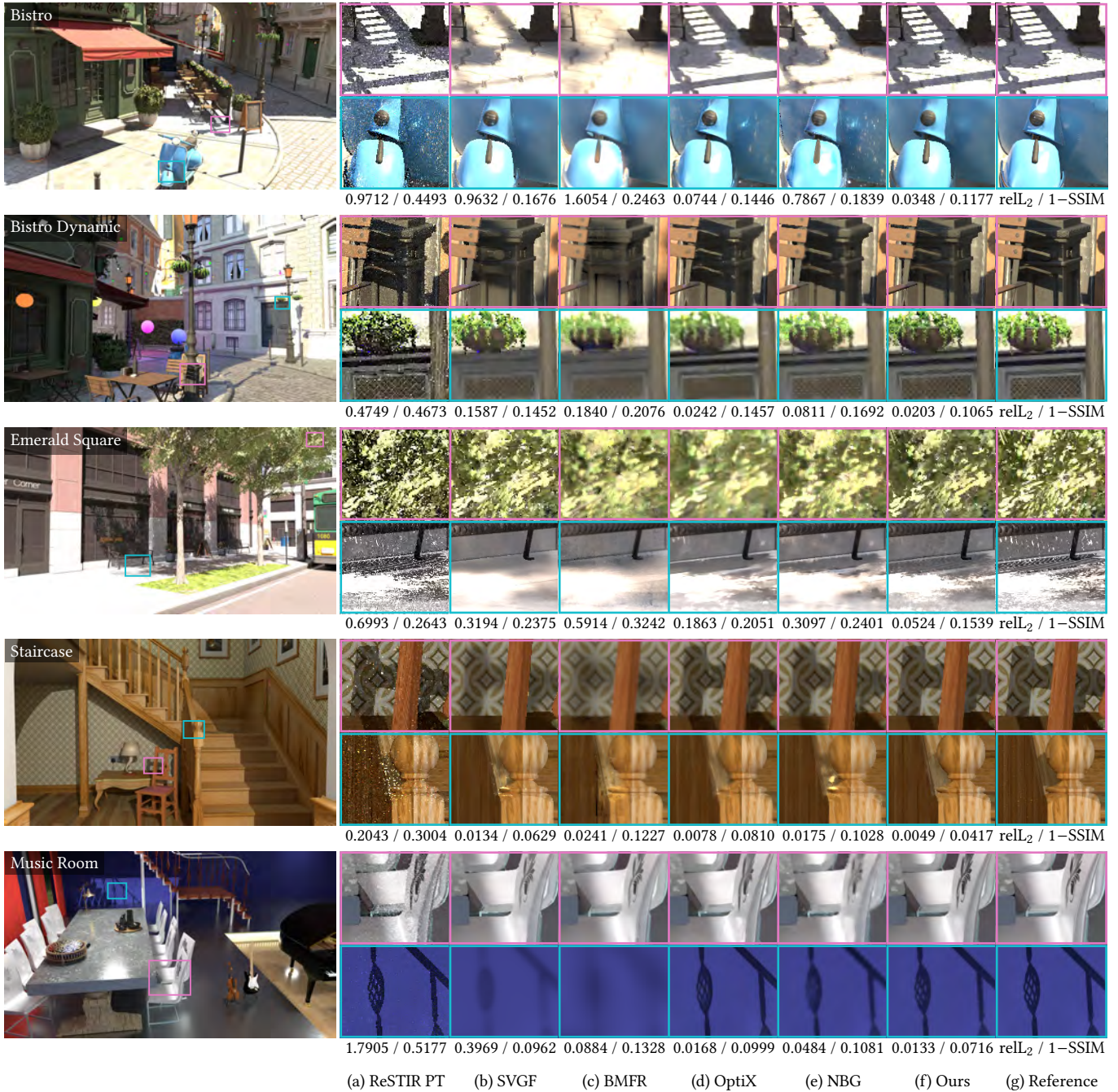
Fig. 6. Comparisons with classical methods (SVGF and BMFR) and supervised learning techniques (OptiX and NBG) for the unbiased input (ReSTIR PT). SVGF (b) and BMFR (c) preserve geometric edges due to the use of G-buffers, but they tend to blur edges introduced by illumination changes, such as shadows. OptiX (d) and NBG (e) maintain such complex edges more effectively than the classical methods, thanks to their use of neural networks. Our method (f) produces visually sharp denoising results while preserving geometric and non-geometric edges, similar to the supervised methods. However, this capability is achieved through a different learning strategy, i.e., online learning, without the need for external training datasets. All images are from the 100th frame of each animated sequence. 3D models courtesy of [Lumberyard 2017] (BISTRO and BISTRO DYNAMIC), [Nicholas Hull and Benty 2017] (EMERALD SQUARE), and Wig42 (STAIRCASE).
